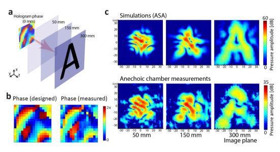
**Figure 3.** Experimental results of the holographic reconstruction of a letter 'A'. (a) The desired pattern to be reconstructed at the depth of 300 mm. (b) The ideal phase pattern designed with GSW method and the actually measured phase pattern immediately behind the hologram. (c) The simulated field patterns (amplitude) at three representative depths compared to those actually measured.
