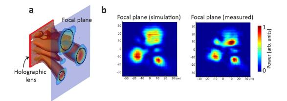
**Figure 4.** Experimental results of the holographic lensing of three circular spots of different diameters. (a) Illustration of the multiple focus lensing with the holographic lens. The isosurface of power and the projected power pattern on the focal plane (300 mm) is calculated with FEM-based full wave simulation. The three dashed circles with different radii are the designed focal spots. (b) The simulated and measured power distribution patterns at the depth of 300 mm.
