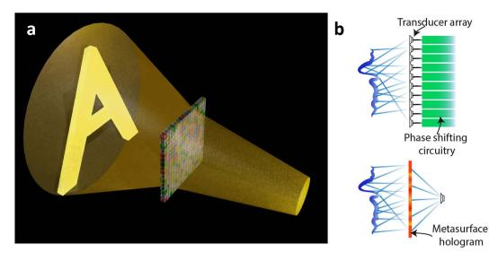
**Figure 1. Schematic of holographic rendering with an acoustic metamaterial-based hologram.** (a) A schematic showing the holographic rendering of a letter 'A' with the passive metamaterial-based hologram. (b) Comparison between holographic rendering with an active phased array and a hologram made of metamaterial-based passive phased array, which eliminates cumbersome phase-shifting electronics and a large number of transducers.
